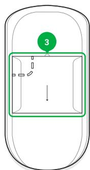
3 - SmartBracket attachment panel (perforated part is required for actuating the tamper in case of any attempt to tear off the detector from the surface).
